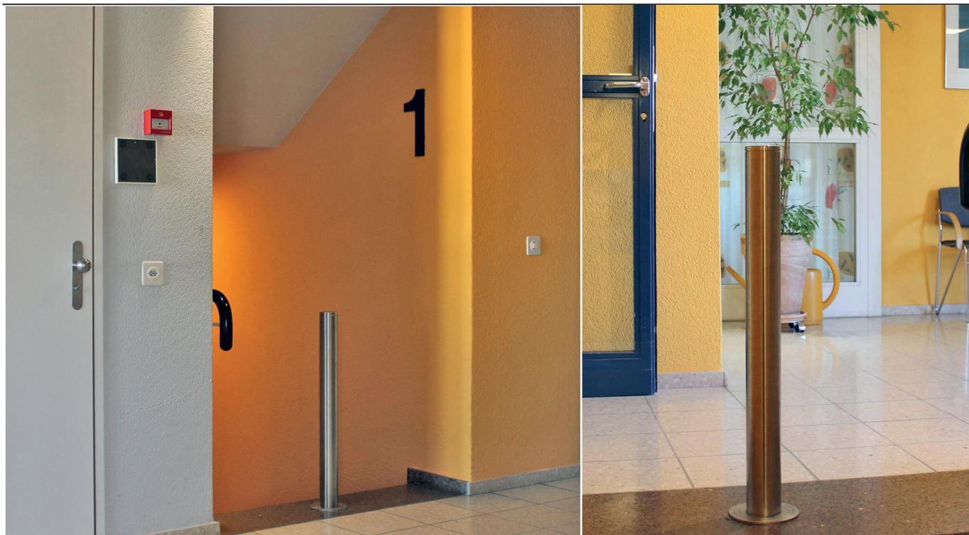
The removable stainless steel indoor bollard is the flexible barrier for public indoor spaces. Developed for protecting wheelchairs from stairs in fairs, shopping centres, airports, museums or nursing homes, it requires a limited installation depth in the floor of only 8-10cm. Indoor spaces can thus be elegantly divided or secured. When the bollards are temporarily removed no opening remains in the floor, so there is no risk of tripping.
